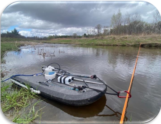
Flow measurement Hall road using Sontek S5 unit (high water)
