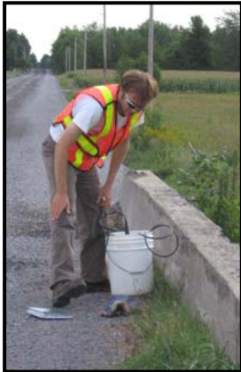
SNC staff taking a reading from a multi-probe while surface water sampling.
