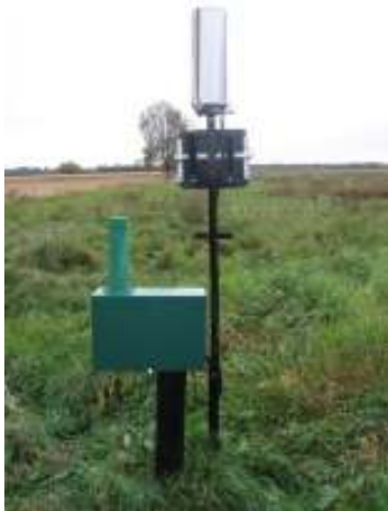
Provincial Groundwater Monitoring Program well set-up.
