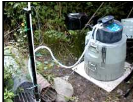
Figure 4: Automated sampler set-up to sample flow from the tiles for the WEBS – controlled drainage BMP.
